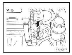
Use the engine oil dipstick to check the oil level. The dipstick's handle will be a yellow ring. See "Engine Compartment Overview" in this section for the location of the engine oil dipstick.
